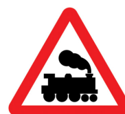
Level crossing without barrier
